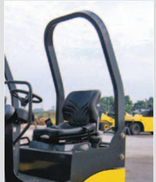
Vibration isolated operators platform minimizes operator fatigue. Standard ROPS with safety seat belts.
