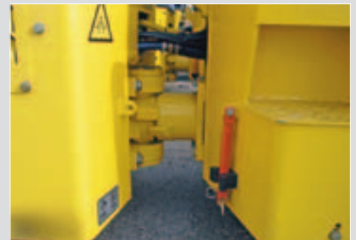
Bolt-on center-joint, with standard crab steer off-set, provides long life and ease of repair.
