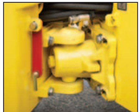
Maintenance free bolt on articulated / oscillating joint.
